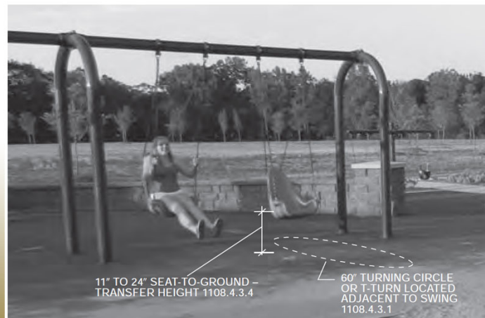
Figure C1008.4.3.1 ACCESS TO SWINGS
